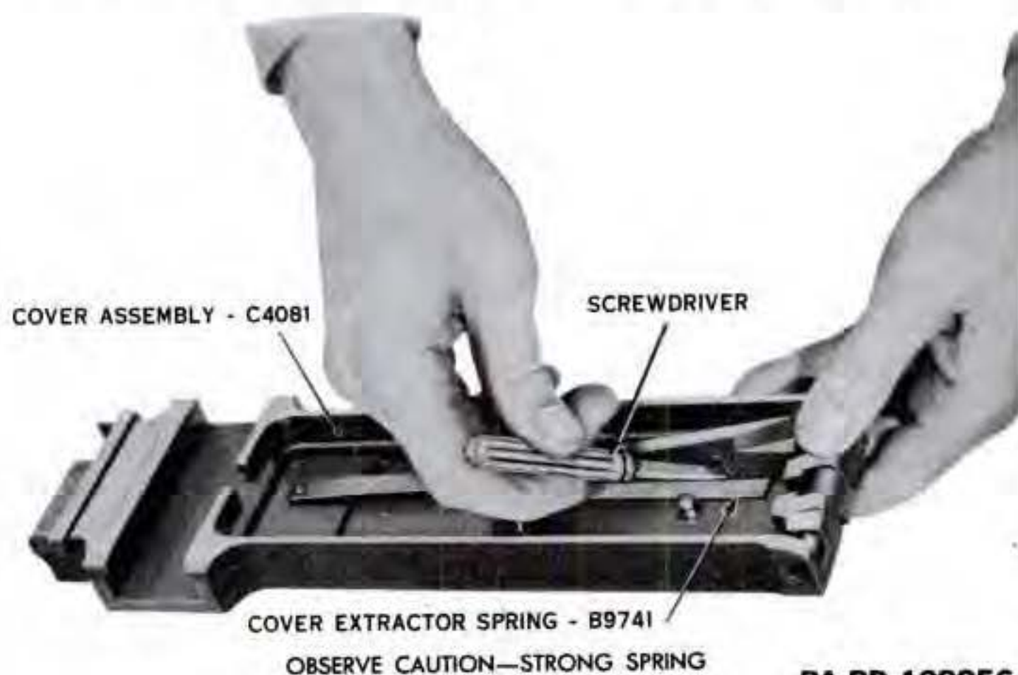
Figure 98. Removing cover extractor spring.
