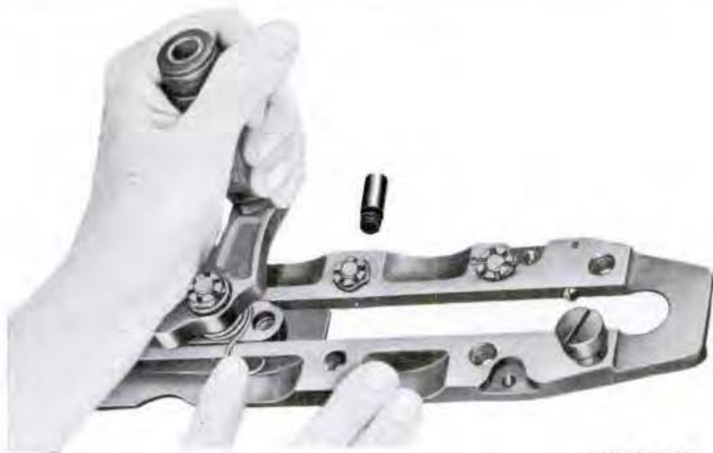
Figure 116. Rotating lever with loop end of spring caught and held over shoulder on bracket.
