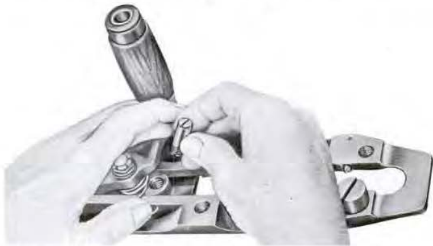
Figure 117. Lever rotated to clear stop hole in slide, and lever and spring held preparatory to screwing stop into slide.
