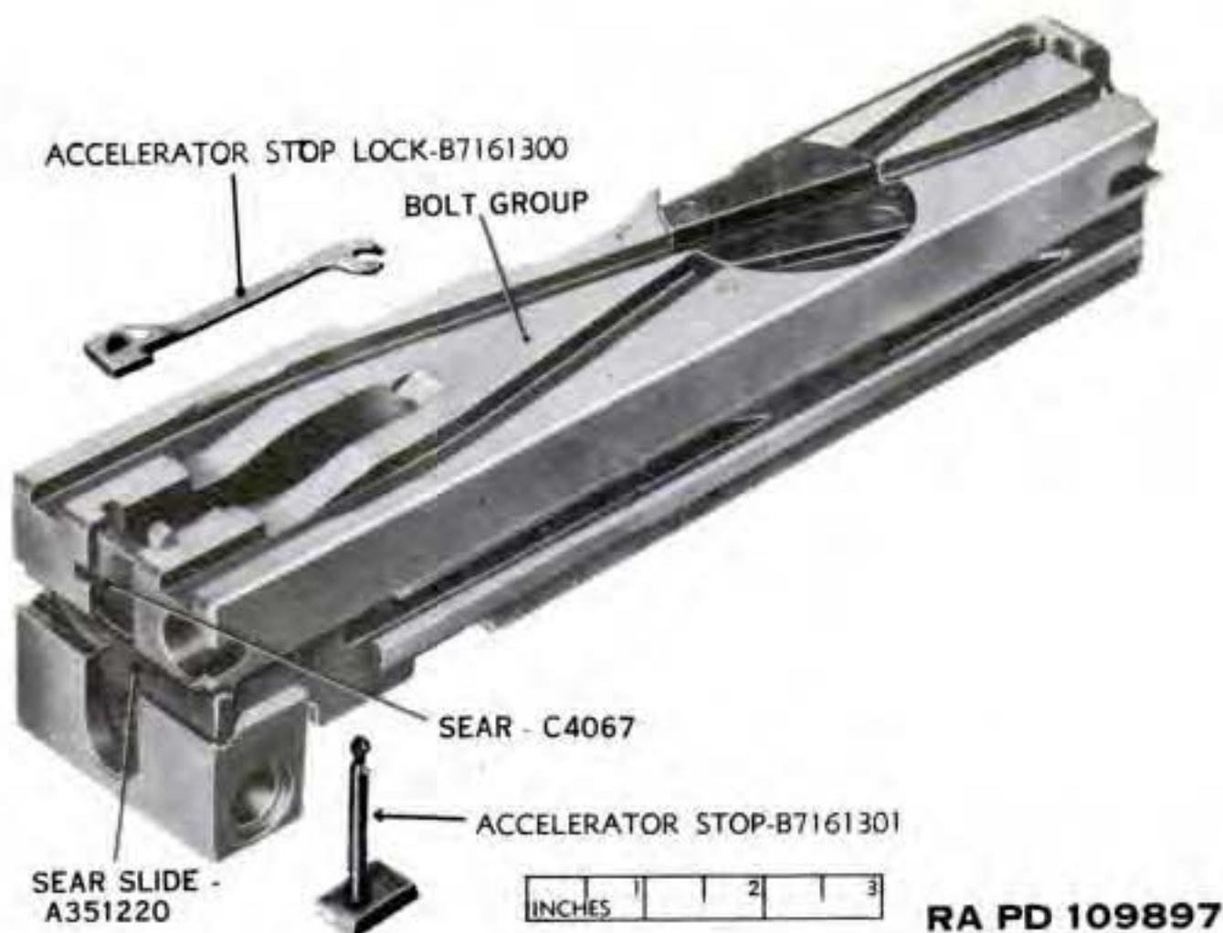
Figure 7. Accelerator stop and lock—exploded view.
