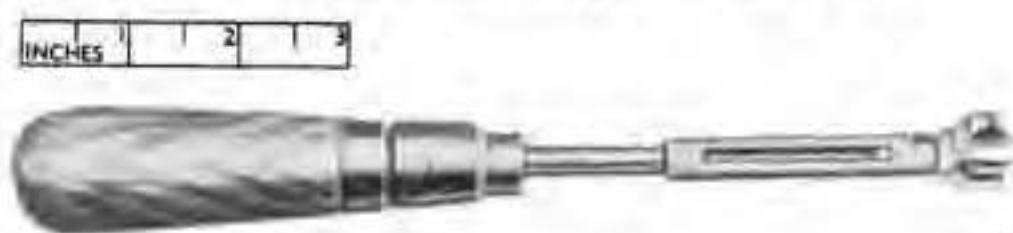
Figure 36. Firing pin spring removing tool.
