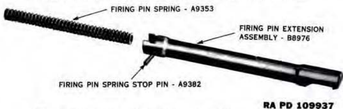
Figure 80. Firing pin extension assembly—exploded view.
