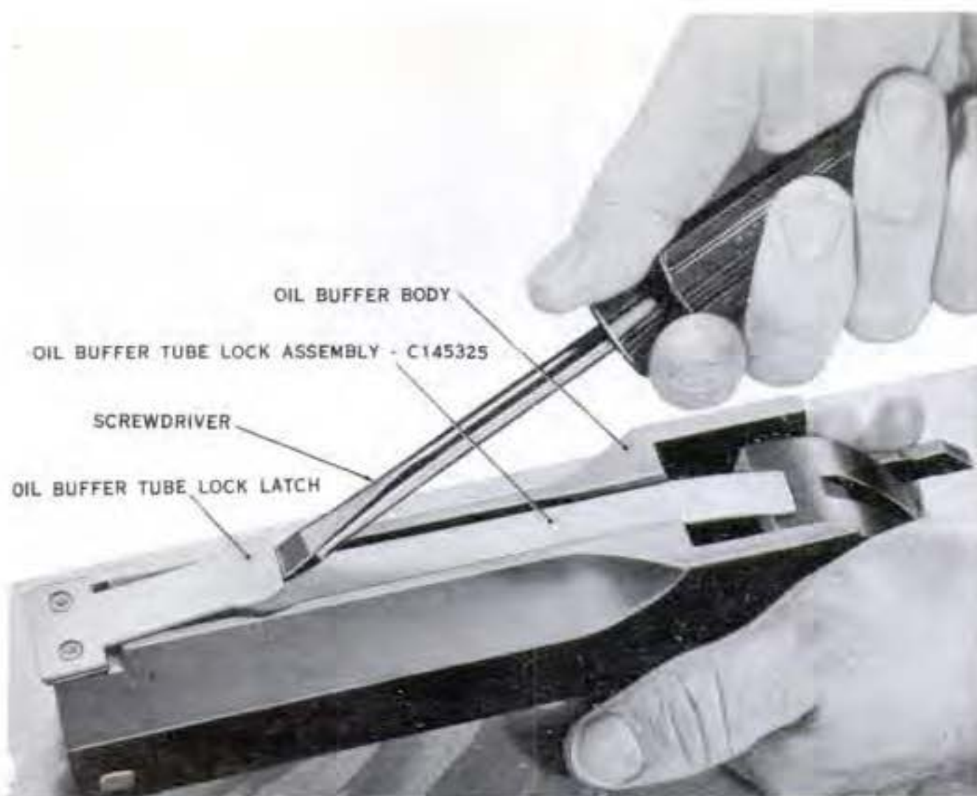
Figure 86. Disengaging tube lock latch from oil buffer body.
