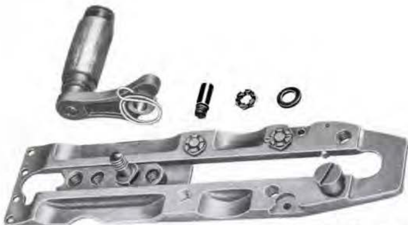
Figure 114. Retracting slide lever spring assembled to lever.
