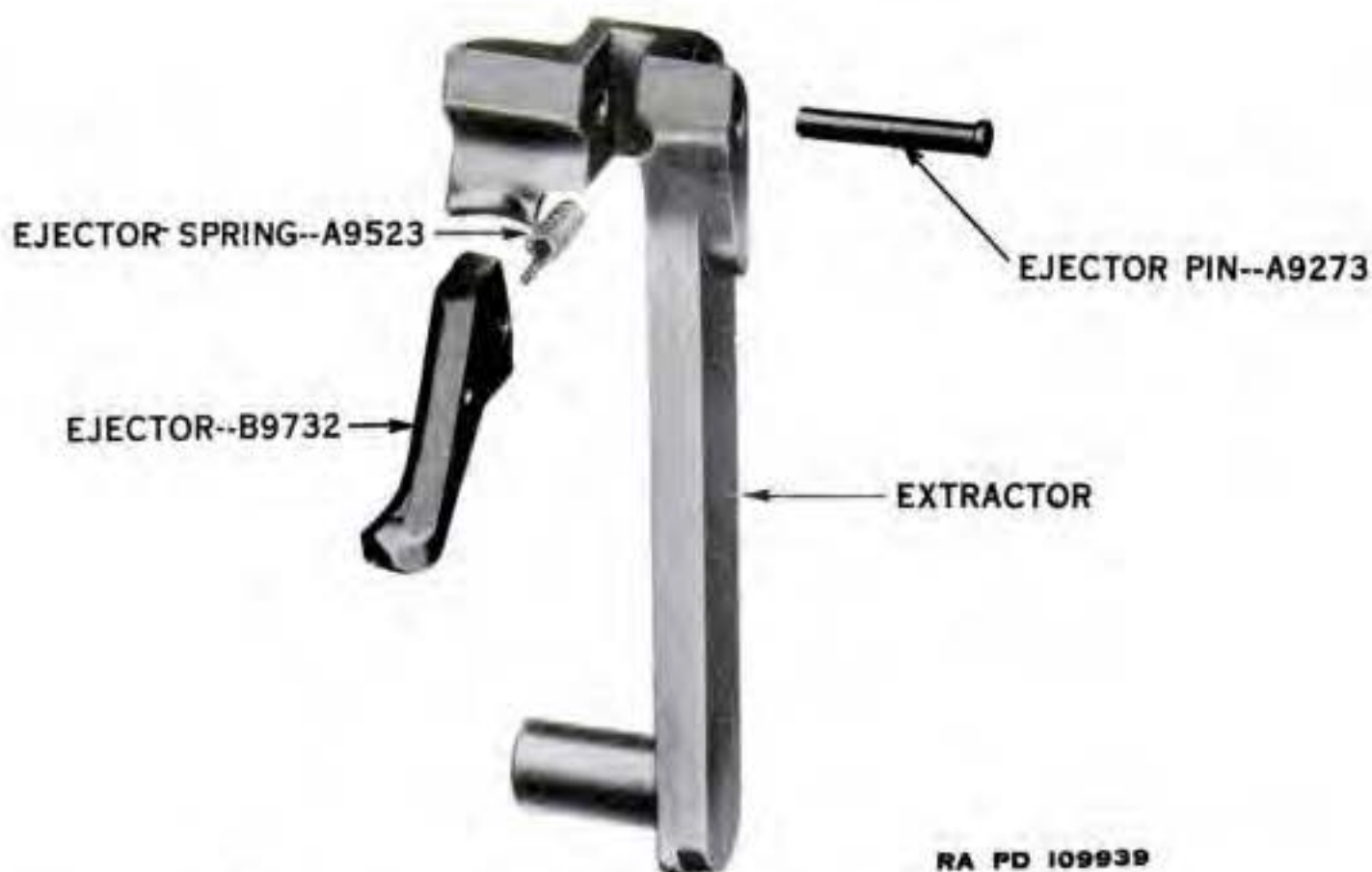
Figure 75. Extractor assembly—exploded view.
