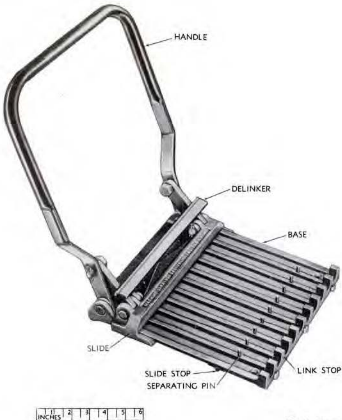
Figure 38. Link-delinking machine, cal..50, M7.
