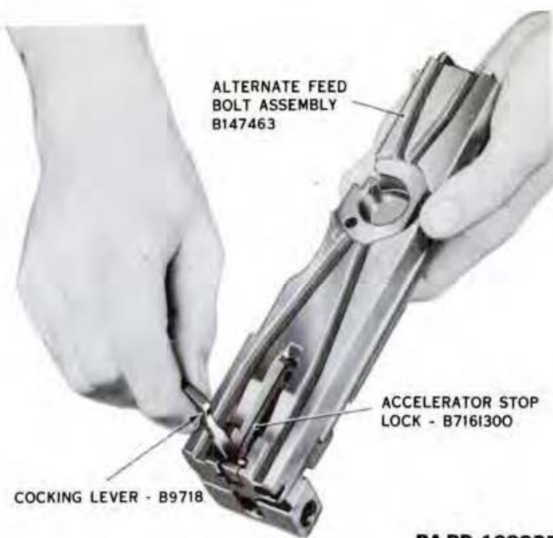
Figure 77. Removing accelerator stop lock.
