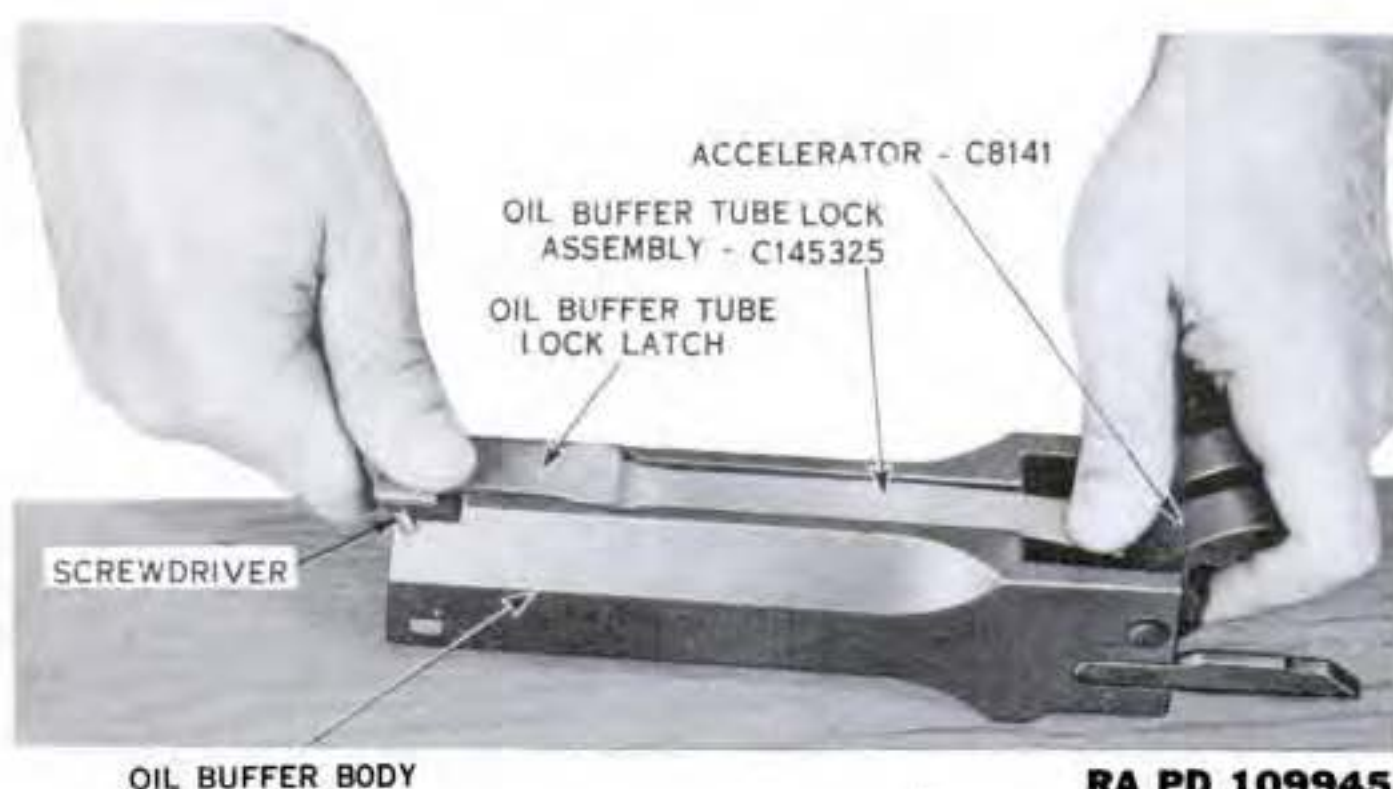
Figure 87. Removing oil buffer tube lock assembly from oil buffer body.
