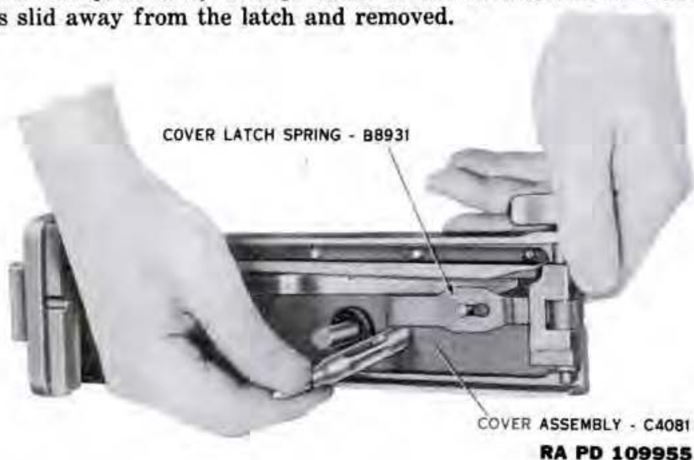
Figure 97. Removing cover latch spring.
