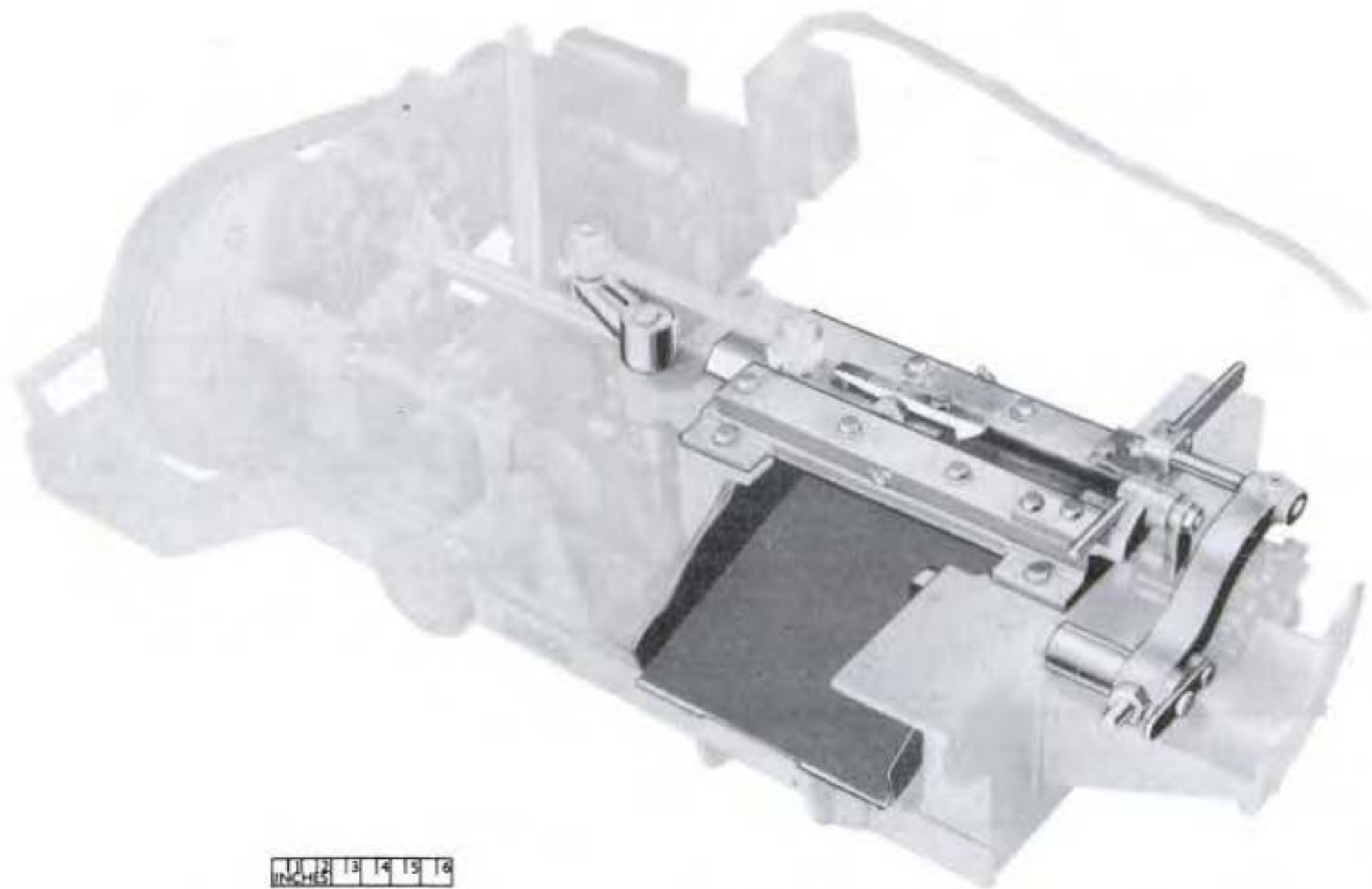
Figure 40. Delinking attachment, cal..50, M7, assembled to powered linking machine, cal..50, M5.
