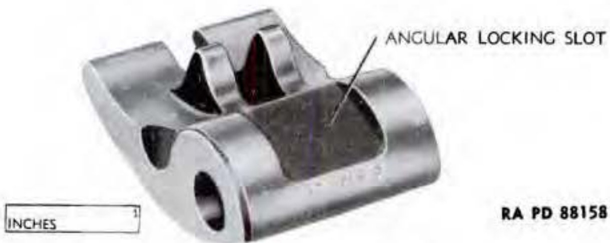
Figure 10. Accelerator with angular locking slot.
