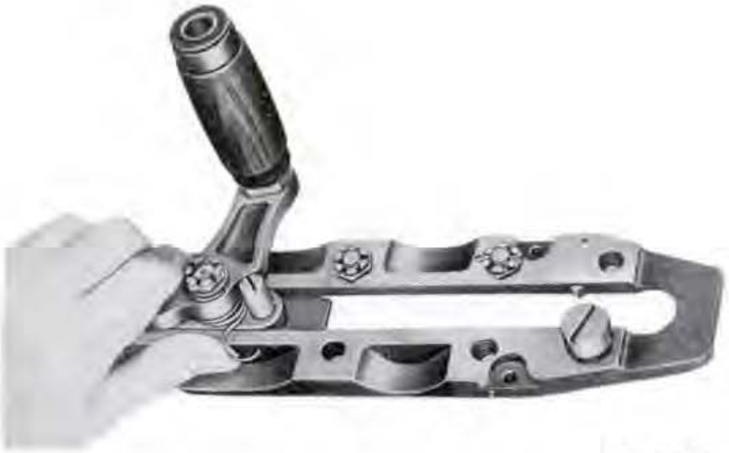
Figure 118. Releasing loop of spring from shoulder of bracket.
