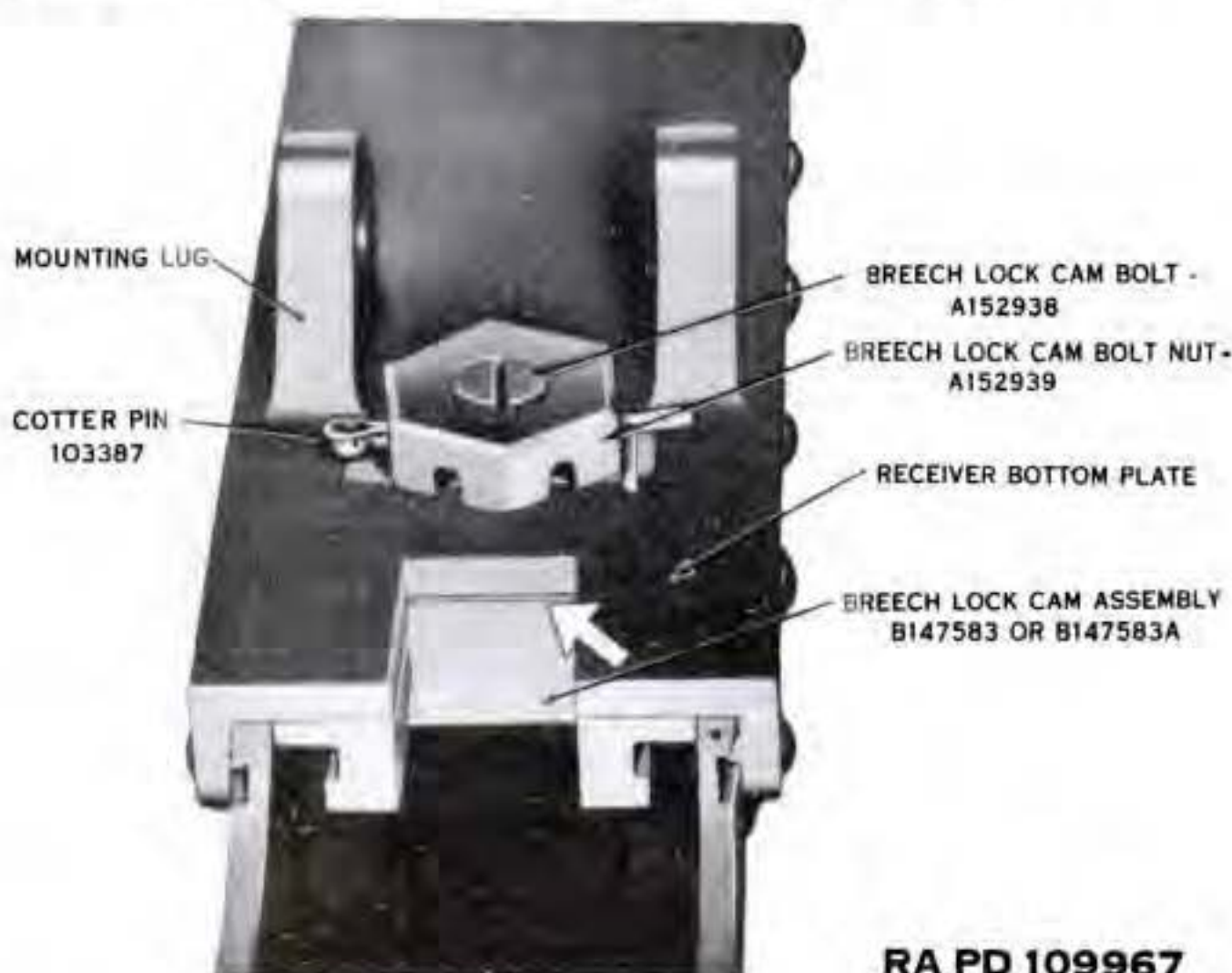
Figure 109. Measuring point for clearance of breech lock cam.
