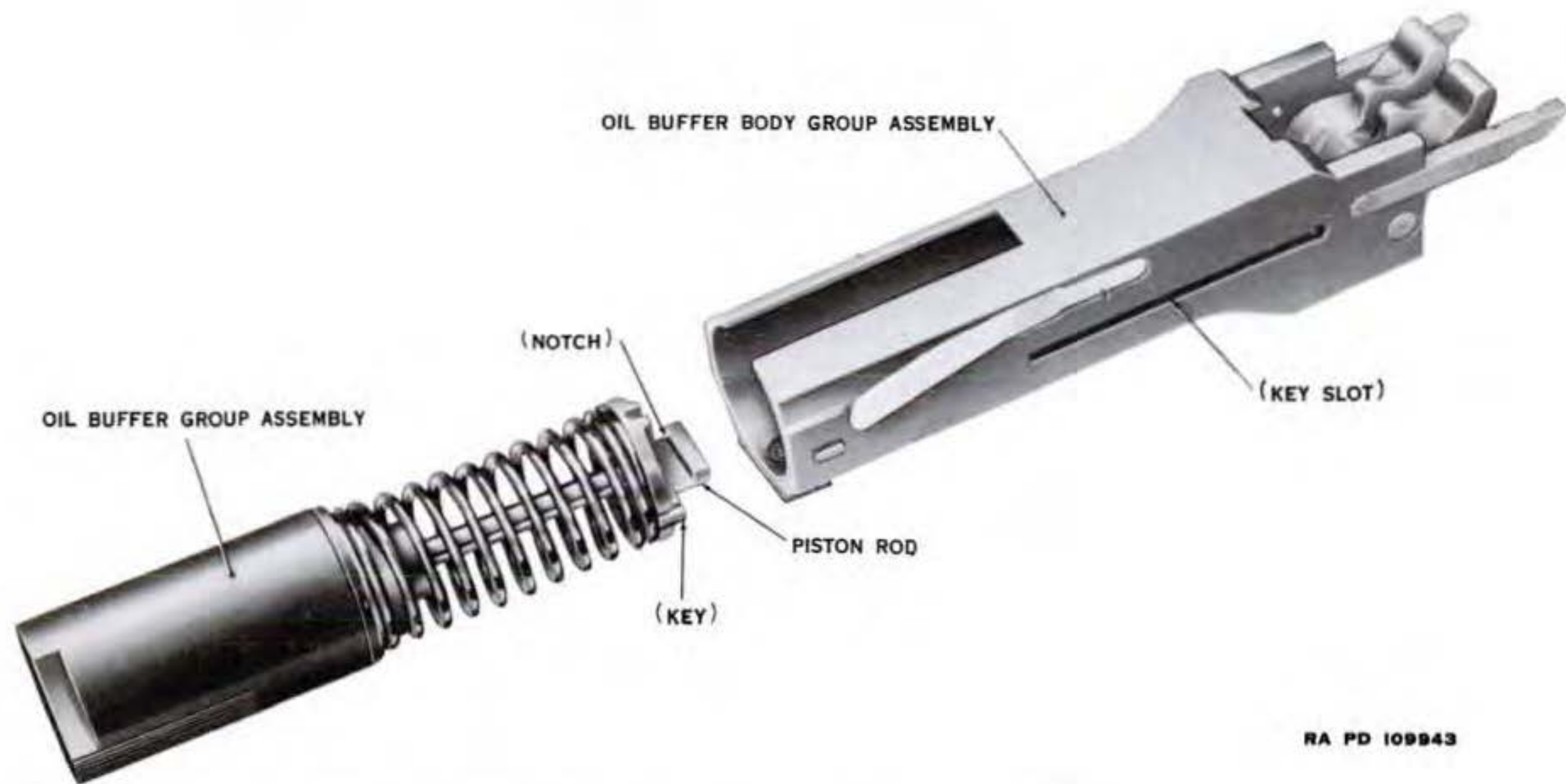
Figure 85. Oil buffer group assembly removed from oil buffer body group assembly.
