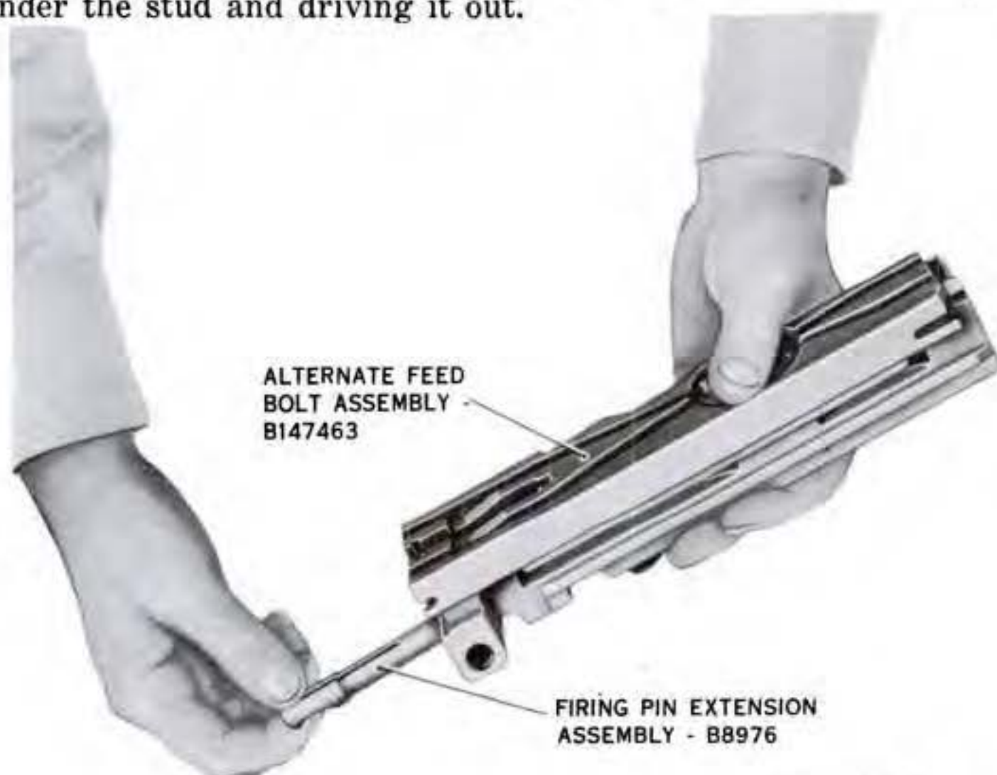
Figure 78. Removing firing pin extension and firing pin.
