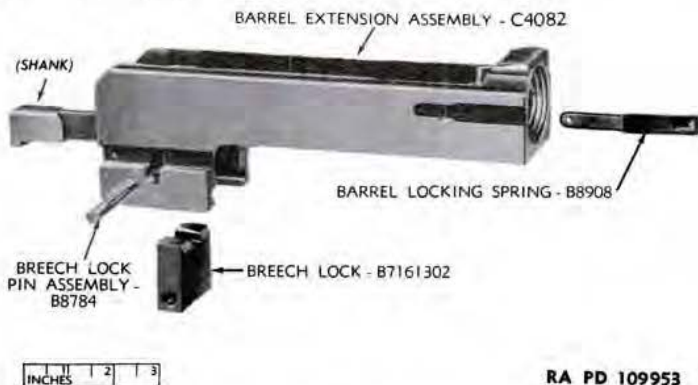
Figure 95. Barrel extension group—exploded view.
