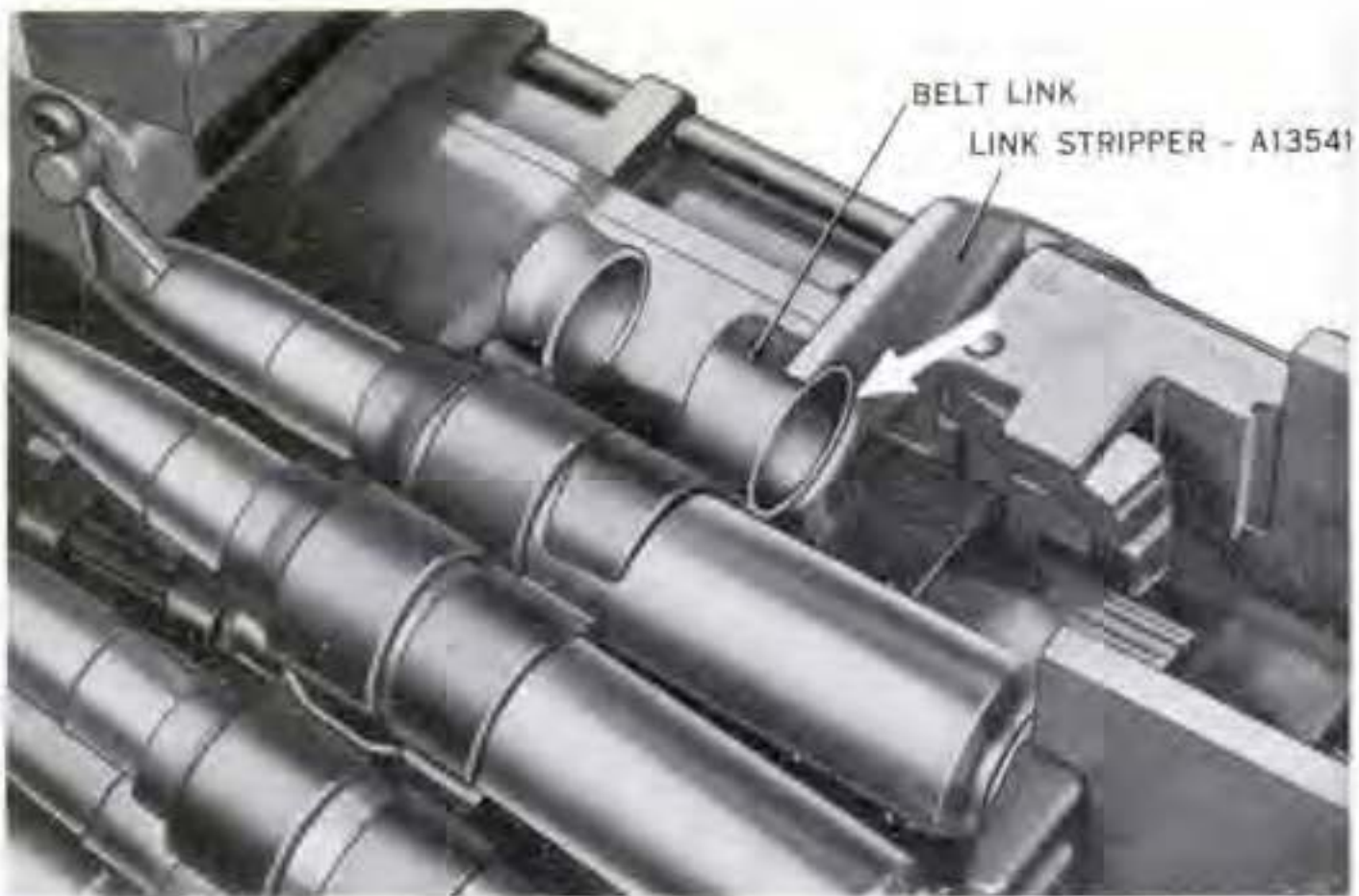
Figure 63. Link caught in link stripper.
